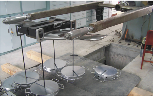
图 4 双天平加载方案 Fig. 4 Loading scheme for the twin balances
