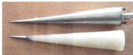
图1 5°钢制和非金属材料尖锥模型 Fig. 1 5° stainless steel and nonmetal sharp cone model
