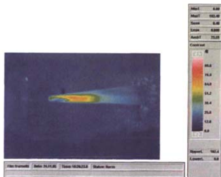
图4 5°非金属尖锥模型红外热像测量结果 Fig. 4 5° sharp cone nonmetal model test results using infrared thermo-graphical technology
