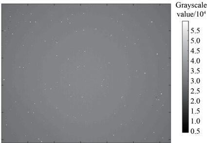
图2 黑体均匀辐射下中波红外相机采集到的原始灰度图像 Fig.2 The original grayscale image obtained by the midwave infrared camera under uniform blackbody radiation
