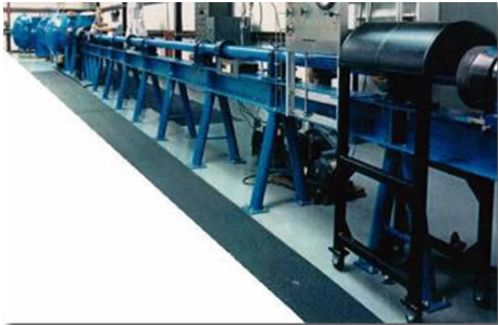
图 2 HVIT 实验室二级轻气炮 Fig. 2 HVIT's two stage light gas gun
