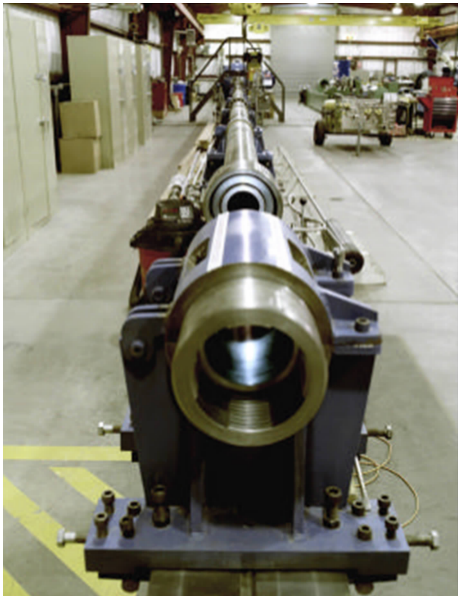
图 3 25.4mm 口径二级轻气炮 Fig. 3 25.4mm caliber two stage light gas gun
